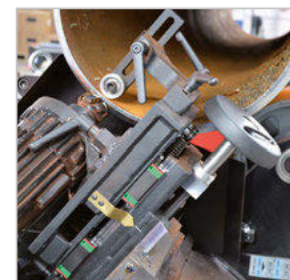
Optional Oval Pipe Tracking Attachment allows out of round pipe beveling
