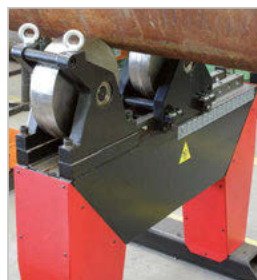
Optional heavy-duty pipe support with 11-ton capacity
