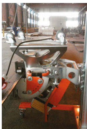
Rotates 180 degrees for bottom side bevel.
