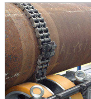
Adjustable chain (ø 8" - 40") ensures positive axial rotation
