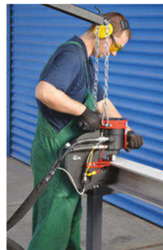
Overhead Support for Punch SM-ZUR-0517-15-00-00-0 Integrated overhead boom support allows for easy manipulation of punch and power pack as single unit.
