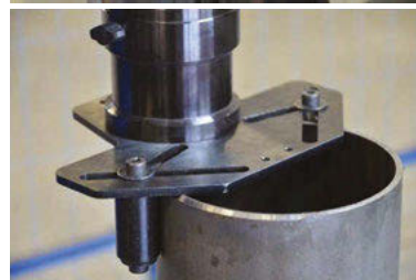
Pipe beveling attachment ID \geq 110 mm OD \geq 150 mm
