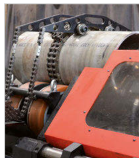
Clamping device for short pipes of 15-3/4" - 32-11/16" length
