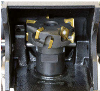
Mono block milling head, with 10 indexable inserts.
