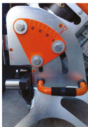
Infinitely adjustable angle between 15 and 50 degrees
