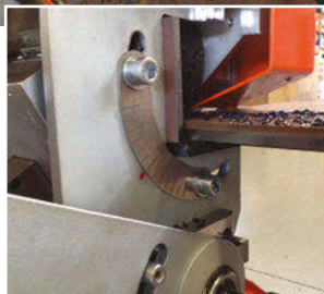
Rapid 180° inversion for bottom side bevel
