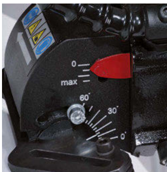
Continuous angle adjustment from 0 to 60 degrees.
